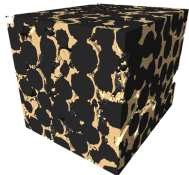
3D image of biofilm (gold) in a packing of beads (black) obtained using X-ray tomography
