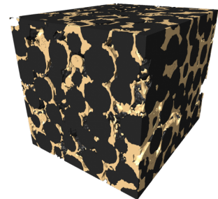
3D distribution of biofilm (gold) in a packing of beads (black). Image obtained using X-ray microtomography.
